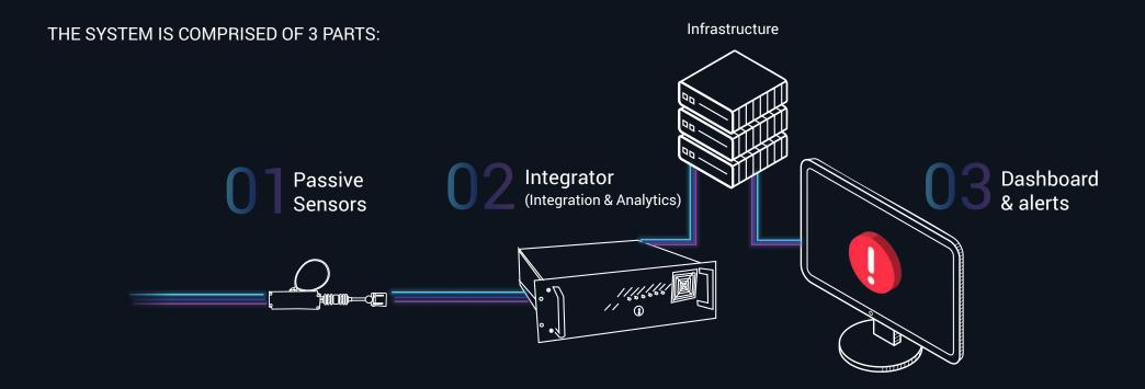
The Fibersafe Integrator collects, and processes data generated by a large number of sensors, enabling remote monitoring of large areas with relative ease while minimizing cost and maximizing resources. Fibersafe Integrator retain large coverage, long-distance monitoring without
