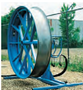
50" (1,270 mm) diameter capstan on Remote Mounting Stand.
