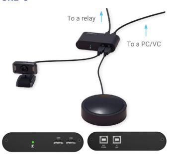
A USB kill switch controlled by a relay, designed to shutdown peripherals in meeting rooms or any other USB device, to be controlled by a room control system.
