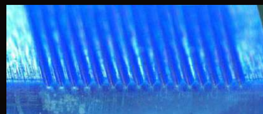
Glass deposition on V-groove
