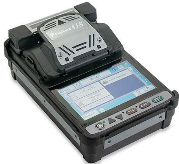
Picture 1. a Splice machine for the house connect
